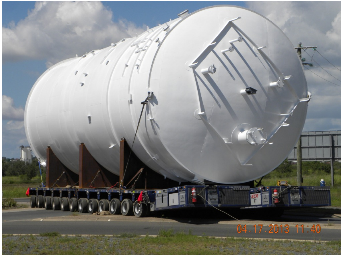
The Amine Surge Tank
