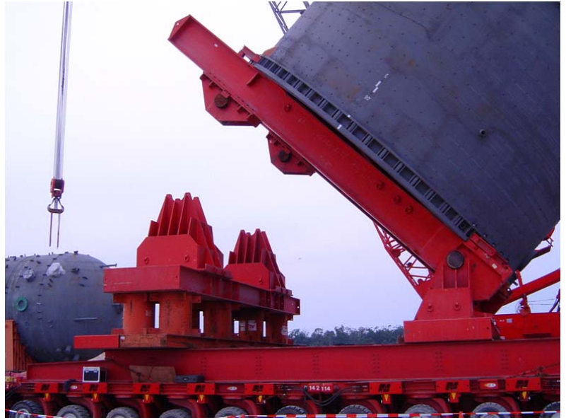
3000t Tailing Frame Capacity 3000 tonnes
