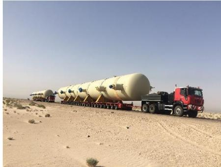
ALE has transported two LPG storage tanks 600km from Umm Qasr Port to Badra Oil Field in Iraq - the largest cargo that has ever been transported this distance in Iraq.
