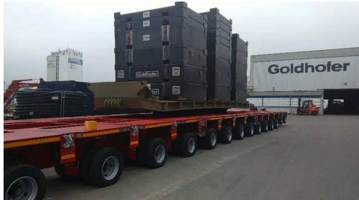
ALE has expanded its global fleet of trailers and invested in the latest range of widening trailers that can be mechanically widened from 3m up to the desired width for the project.
