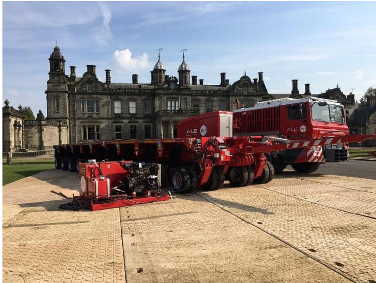
ALE has expanded its global fleet of trailers and invested in the latest range of widening trailers that can be widened to 4.3m whilst loaded, making these the only trailers of their kind in the UK.
