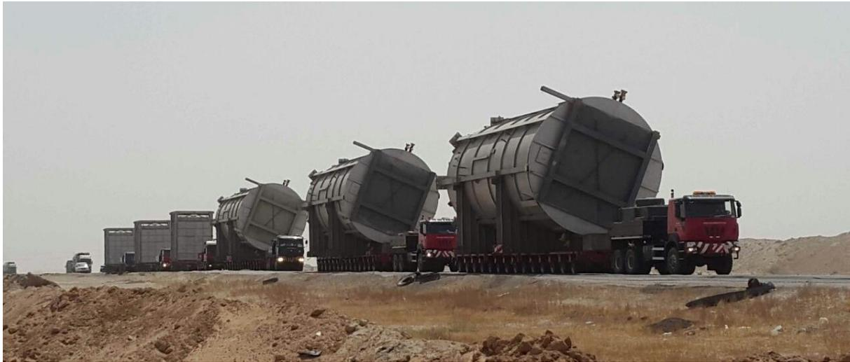
ALE is progressing with the DGS Zubair Oil Field Project and has transported 16 Out of Gauge (OOG) items.
