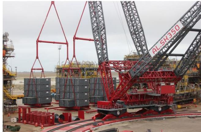
The world's largest capacity land based crane, the AL.SK350, has been rigged for the first time and successfully load tested. The crane was load-tested in preparation of its first lifts on a FPSO (Floating Production, Storage and Offloading) module integration project in Brazil.
