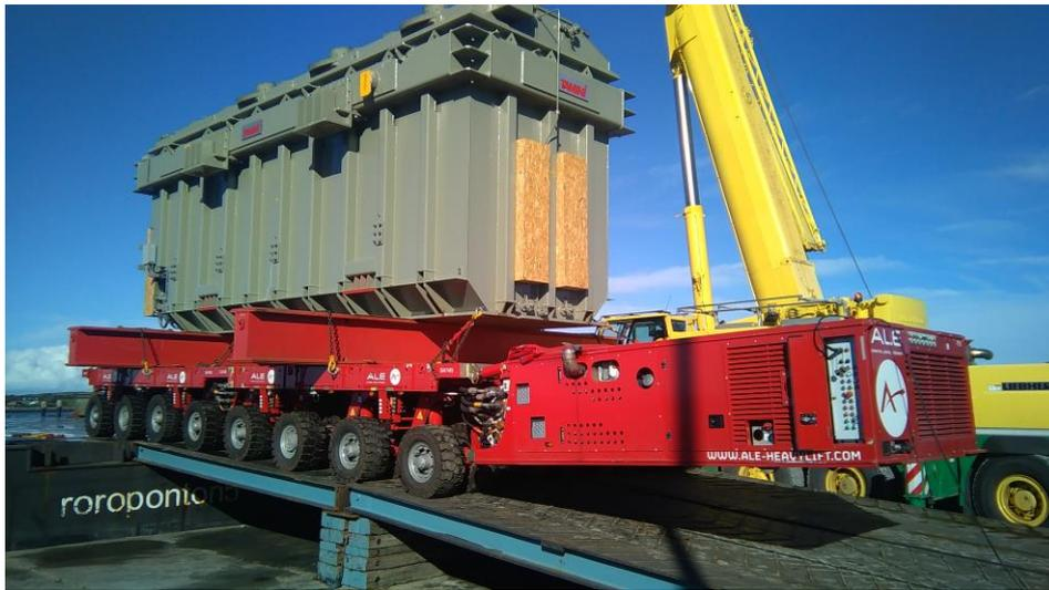
ALE has delivered a transformer, weighing 345t, to a power station in County Claire, Ireland. This is the largest transformer ever to be transported in Ireland.
