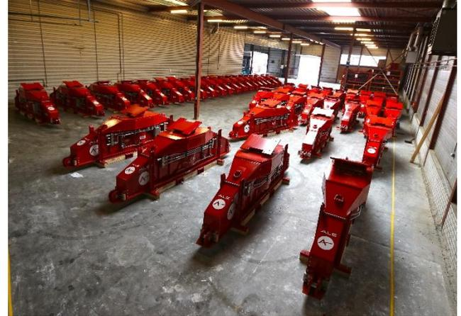
ALE has designed and built a new self-propelled skid system, the SS800, with 800t capacity skid shoes. In total, 48 800t skid shoes, 12 83t push/pull units and 190 5m skid tracks have been built.
