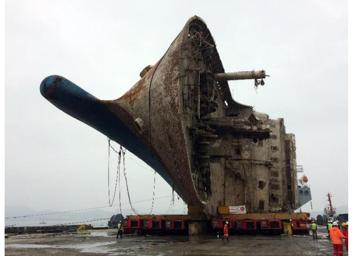
ALE has completed the load-in of the Sewol ferry using a record-breaking number of SPMTs, as part of a complex salvage operation in the East China Sea in April. At 17,000t, this is the heaviest piece ever to be transported by SPMTs.
