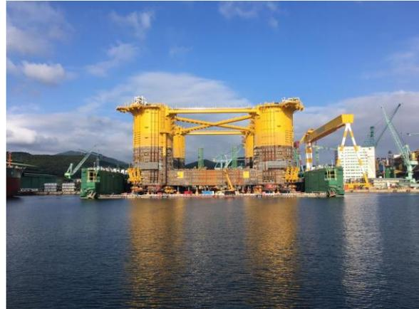
ALE has performed their heaviest-ever load-out operation by hydraulic skidding when performing the back skidding and load-out of an Appomattox hull, weighing over 40,440t, in South Korea.
