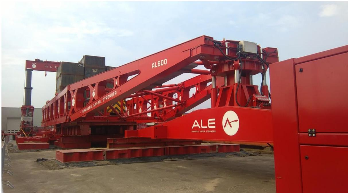
ALE has built a new high capacity girder frame, the AL600. The AL600 will be able to carry loads up to 600t - 100t more than ALE's current largest frame, the AL500.
