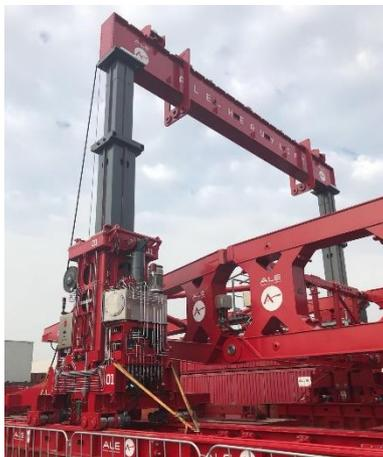
ALE has developed a new telescopic lifting gantry with 1,000t capacity on four towers, the TLG1000. This is the first system in a new fleet of high capacity hydraulic gantries.
