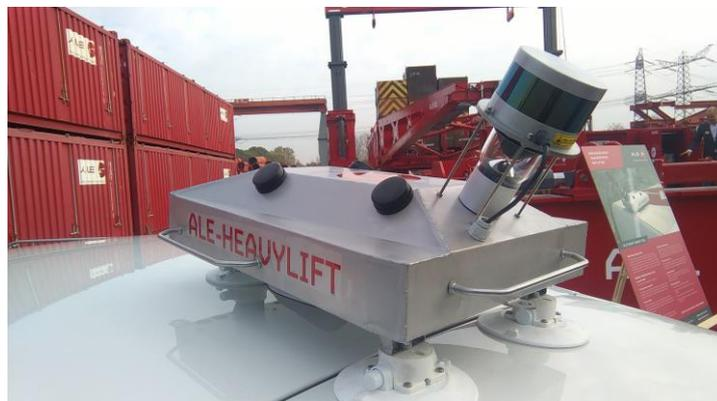
ALE has launched its new Route Survey Tool, which is set to revolutionise the way route surveys are carried out in the heavylifting industry.
