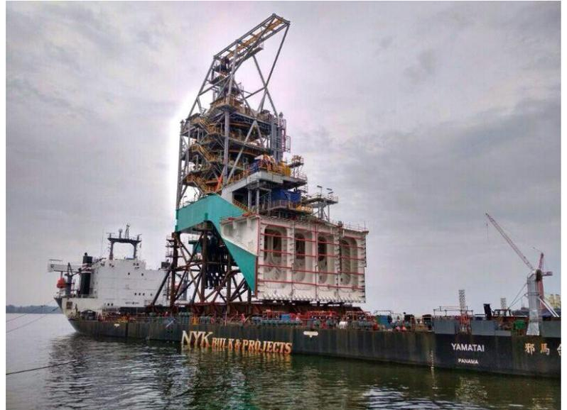
ALE has demonstrated its multi-service capabilities to complete work on a project involving the transportation of a turret mooring system, weighing 3,702t, in Johor, Malaysia.
