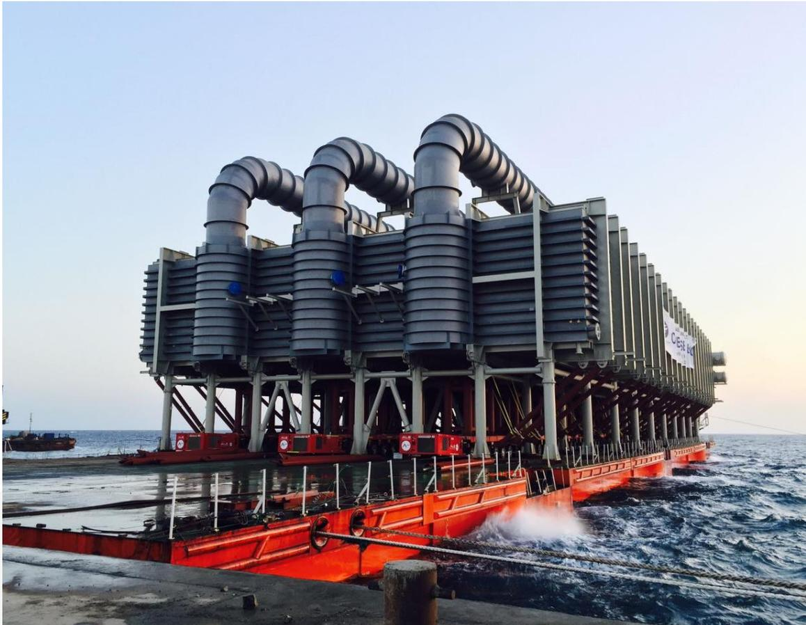
ALE has broken another world record to transport the world's heaviest evaporator, weighing 5,134t, in Saudi Arabia.
