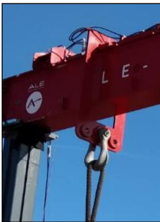
Figure 2 – Hang plate on top of the header beam
