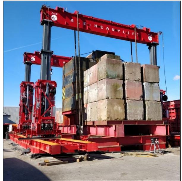
Figure 1 – TLG1000 system during load test
