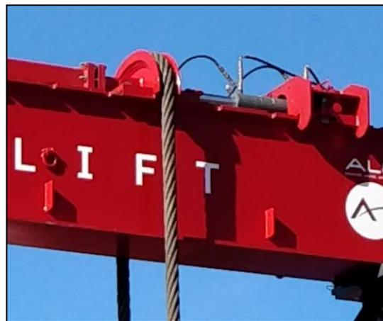
Figure 3 – Wire rope skid on top of the header beam
