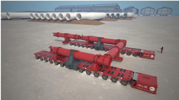
ALE is optimising offshore wind project costs by designing a unique new modular transport frame specialised in carrying transition pieces (TPs) within marshalling ports.
