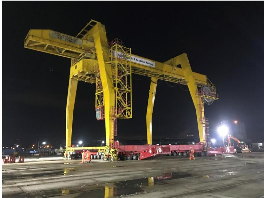
ALE has used its internal engineering expertise to create a special solution that could move a gantry crane, weighing 290t, over live rail lines in the safest way possible.
