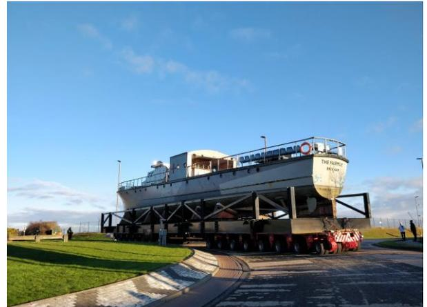
ALE has designed bespoke equipment to complete the jacking, transportation and installation of a fragile Second World War rescue vessel, Rescue Motor Launch (RML) 497, in Hartlepool, UK.
