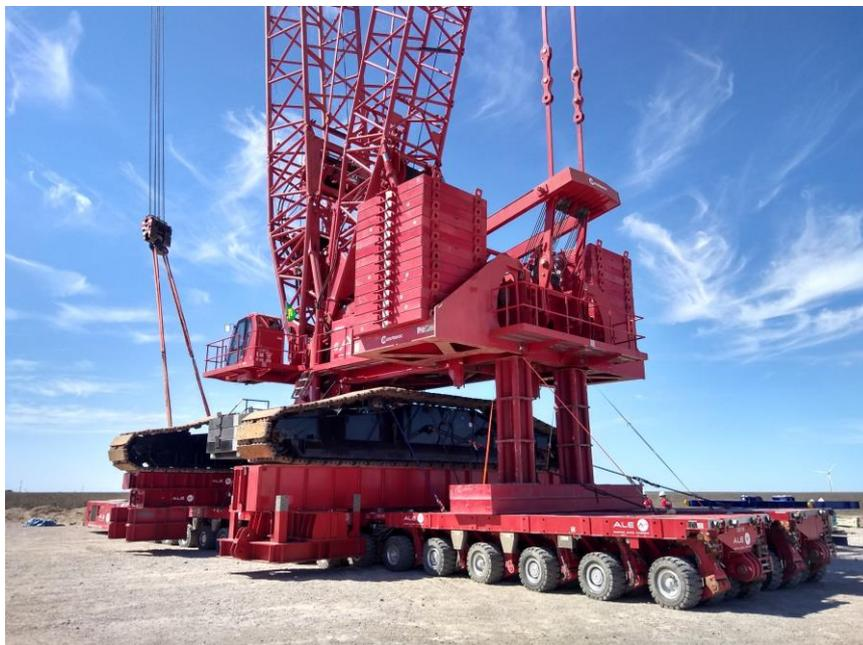
ALE has utilised its innovative methods to adapt a crawler crane, Manitowoc 18000, with SPMTs to significantly reduce the schedule for the Loma Blanca wind farm project in Argentina.
